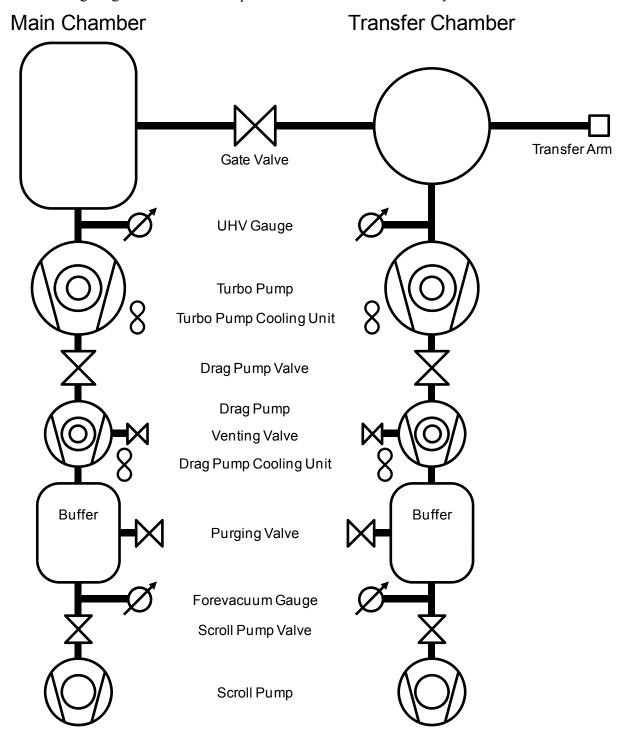
Except for the Gate Valve and the Transfer Arm, each component exists twice. So, there is, e.g., a "Main Scroll Pump" and a "Transfer Scroll Pump".
